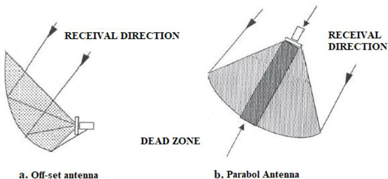
In offset antennas, satellite signal arrives at a certain angle on the antenna, so the focal point of antenna shifts to an area outside the antenna signal receiving surface. Therefore, the LNB does not intercept satellite signals on the antenna and does not cause a dead zone on the antenna. Offset antennas appear to be superior to parabolic antennas with these features, but are not used much above 3 m as they hold too much wind in large antennas.
