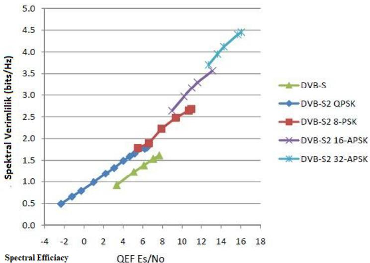
Services and practices offered by DVB-S2 standard cover a much wider range than DVB-S, and it is possible to achieve high bit rates with this standard. DVB-S2 standard, with the increase in H264 and MPEG compression standards, can easily provide the necessary bandwidth for
